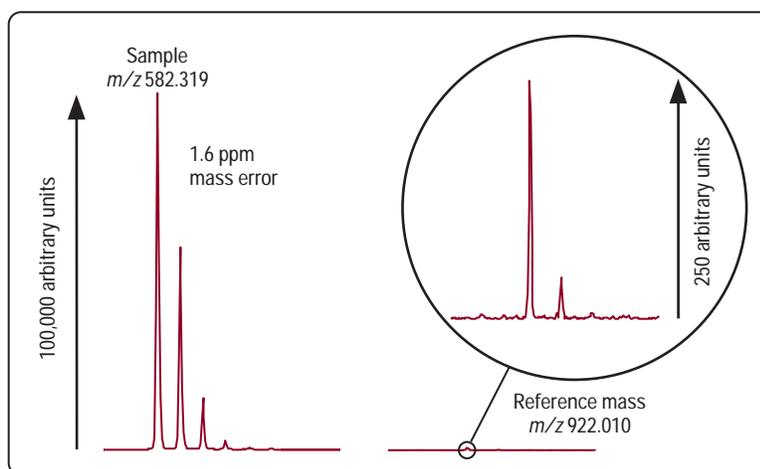
Wide dynamic range ensures that both major and minor components are identified, and facilitates use of an internal standard
