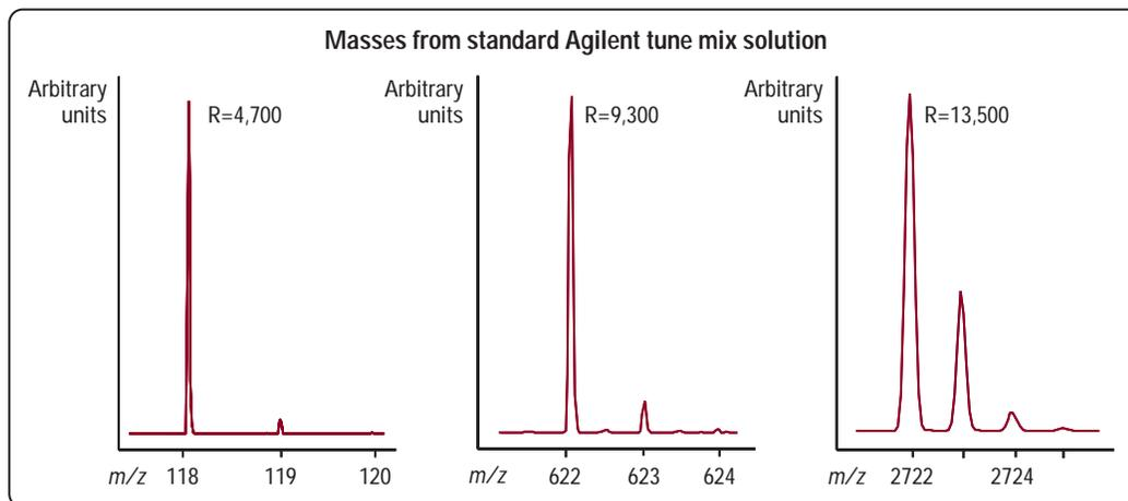
The 6210 TOF's high resolving power ensures the best chance of distinguishing all sample components
