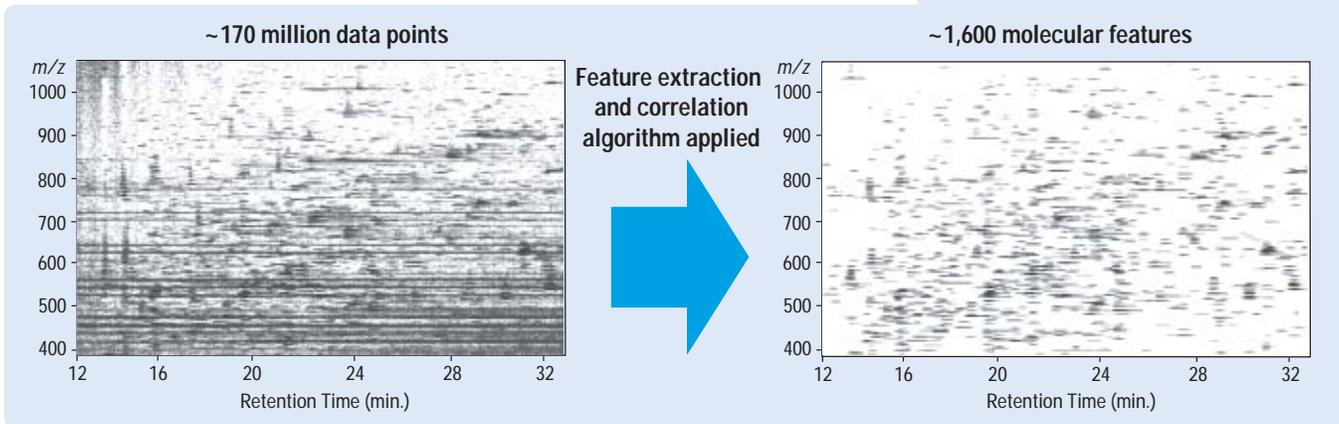
Processing of raw data with the feature extraction and correlation algorithm identifies approximately 1600 compounds out of 170 million raw data points from a sample of BSA spiked with myoglobin. These examples zoom in on a small region of the total data display.
