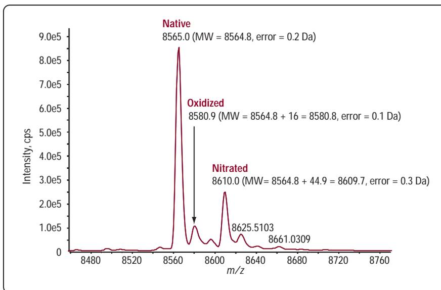
The MassHunter Bioconfirmation software discerns modified forms of proteins, as shown in this deconvoluted spectrum of three major products in a peroxynitrite-treated ubiquitin sample
