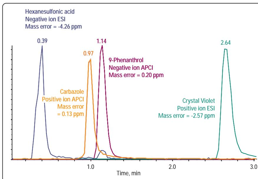
In a single run, a 6210 TOF with spectrum-to-spectrum polarity switching and a multimode ion source identifies four compounds that each respond to a different combination of ionization method and ionization polarity
